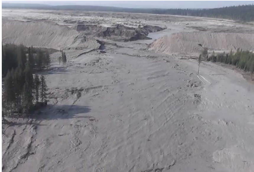
Mount Polley Mine Tailings Impoundment Breach (photo courtesy of Farhan Umedaly, Vovo Productions)
